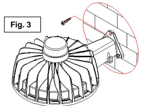
6. Secure power supply inside wiring compartment using 1/2" connector (by others).
