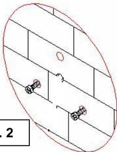
3. Insert two screws (provided) into the two lower-most mounting hole locations, as shown in Fig. 2. Do not tighten the screws fully.
