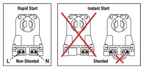
Figure 1. - Non-shunted & Shunted Lamp Holder
