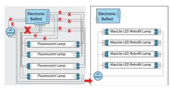
Figure 4. - Retrofit with Three/Four Lamps
