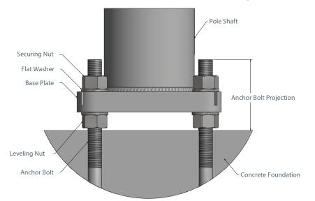
**NOTE:** Do not erect pole without the intended loading attached.
