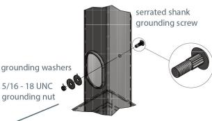
The poles must be hung in order to travel through the powder coat booth. We do this by drilling(2) holes in the pole. The hole at the top is plugged while the hole at the bottom of the pole is utilized as the Grounding Lug.
