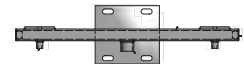
PL-XSB2-B (2 FIXTURES, 1.90 EPA) PL-XSB3-B (3 FIXTURES, 2.60 EPA) PL-XSB4-B (4 FIXTURES, 3.30 EPA) PL-XSB5-B (5 FIXTURES, 4.0 EPA) PL-XSB6-B (6 FIXTURES, 4.75 EPA)
